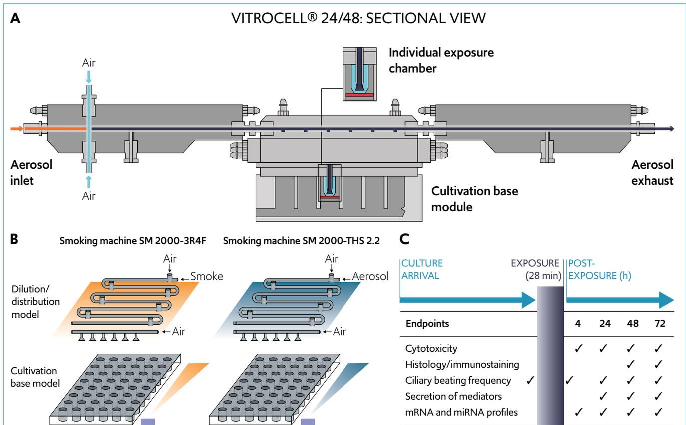
Figure 4 Schematic representations of the VITROCELL® 24/48 exposure system
