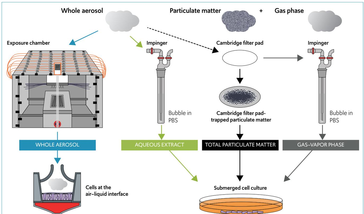
Figure 2 Experimental design for collection of and in vitro exposure to the whole aerosol (WA), aqueous extract (AE), total particulate matter (TPM), and gas-vapor phase (GVP) fractions
