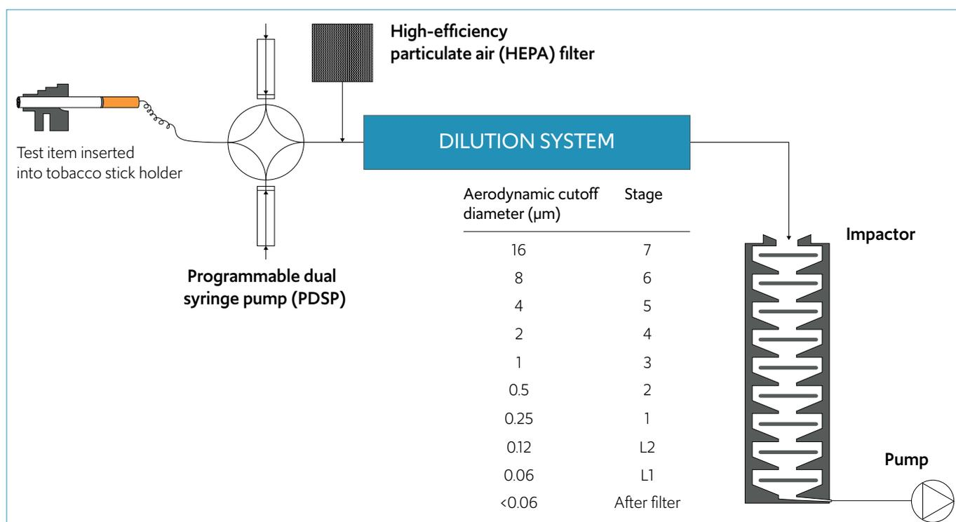
Figure 3 Experimental setup for cascade impactor measurement of particle size distribution
